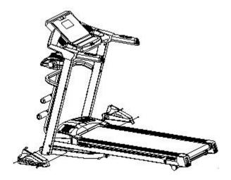
Step VIII: Carefully inspect the fastening of each part of treadmill; start the treadmill at low speed and inspect the flexible rotation of each part of running belt and the tightness of running belt; the non-offset and non-skidding of running belt shall prevail (see the "Daily servicing and maintenance of electric treadmill"). After the inspection, move the treadmill to a proper position for use.
