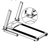
Step III: install display screen: open packing box of the display screen, take out of display screen, correspondingly connect lines on the display screen and the lines on the meter, plug the display screen into the meter, lock it on the meter with four M6×20 hexagon socket head cap screws (with spring washer and flat washer), as shown in the following figure:
