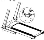
Step III: install display screen: open packing box of the display screen, take out of display screen, correspondingly connect lines on the display screen and the lines on the meter, plug the display screen into the meter, lock it on the meter with four M6x20 hexagon socket head cap screws (with spring washer and flat washer), as shown in the following figure:
