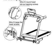
Step V: Carefully inspect the fastening of each part of treadmill; start the treadmill at low speed and inspect the flexible rotation of each part of running belt and the tightness of running belt; the non-offset and non-skidding of running belt shall prevail (see the "Daily servicing and maintenance of electric treadmill"). After the inspection, move the treadmill to a proper position for use.
