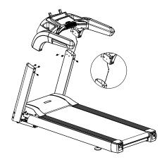
Step IV: Install the decorative elements of upright pole and lower meter: Firstly, fix the decorative elements of left and right upright poles at the treadmill in 6 M8×8 large crossed flat head screw; secondly, fix the decorative elements at lower left and right of the meter on the left and right upright poles below the meter head in 2 M4×8 large crossed flat head screw and 4 M4×10 round head tail-cut tapping screw, as shown in the figure below:
