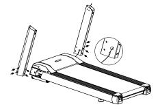
Step III: Install screen: Open the packing box and then take out the screen. Firstly, connect the wire of the screen with that of the meter head in one-to-one way; secondly, insert the screen into the meter head; finally, lock the screen on the meter head in 4 M6×25 hexagon socket head cap bolts (containing shim), as shown in the figure below:
