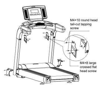
Step V: <u>Install bulkhead and power line</u>: Firstly, plug the installing holes below the left and right upright poles and the meter head with 6 bulkhead; finally, connect the power line with one-piece power switch of the treadmill (note: guarantee the power line is off before connecting the power line, so as to avoid personal injury), as shown in the figure below:
