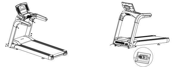
Step VI: Carefully check if each part of the treadmill is tightened. Run the treadmill at the slow speed and check if the each part of the running belt is flexibly rotated and whether the tightness of the running belt is proper. As for the running belt, no offset and sliding will prevail (see "Daily maintenance of powered treadmill"). Move the treadmill to the proper position and then use it after the check is completed.
