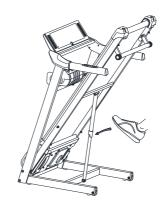
pick up the treadmill frame with hands, stamp the air spring casing so that the air spring can retract into the casing, and slowly set the treadmill level in order. The stamping for air spring casing is as shown in the figure.
